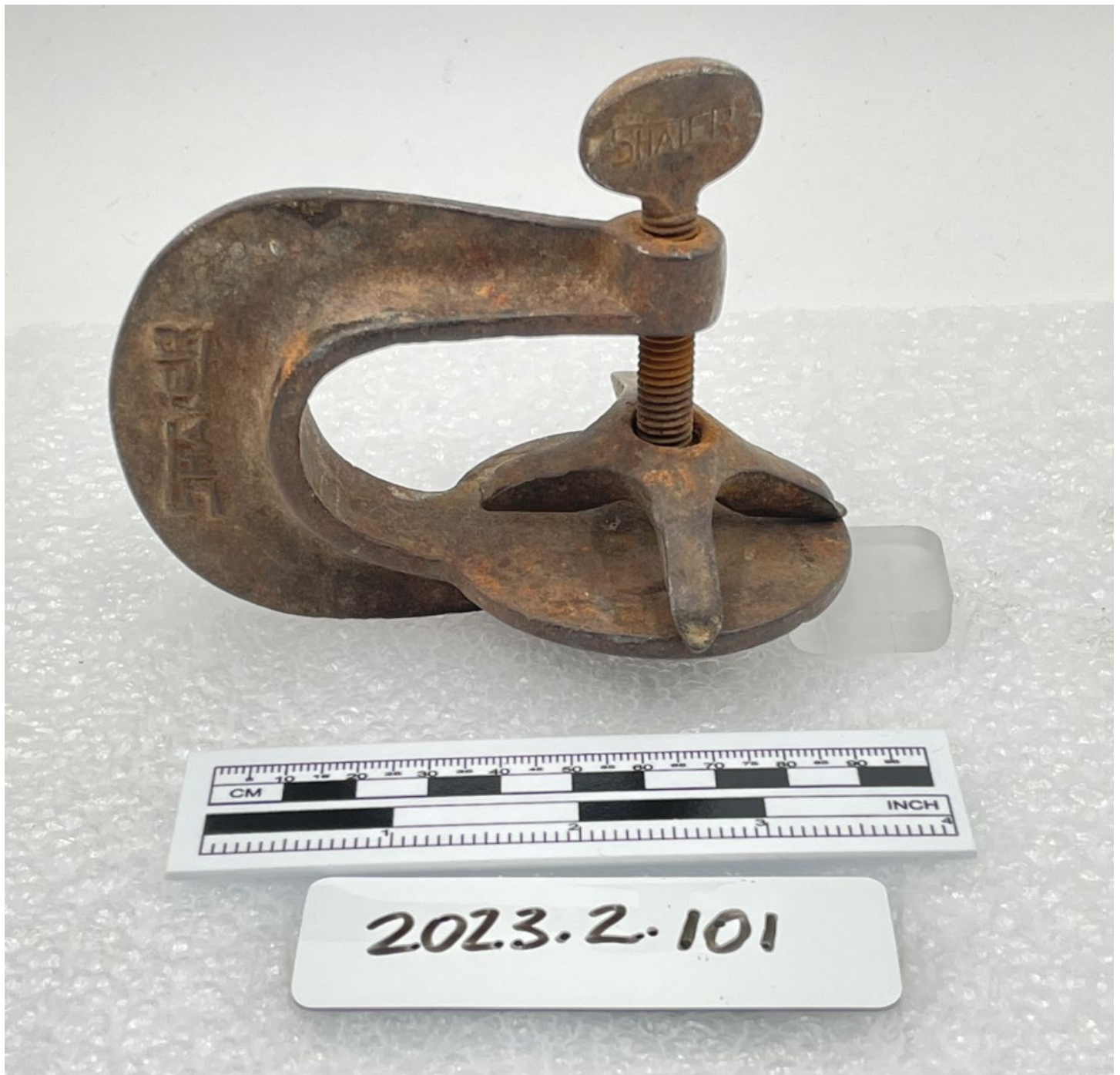
Shaler 5-Minute Vulcanizer, used while patching automobile tires in the 1920s:
